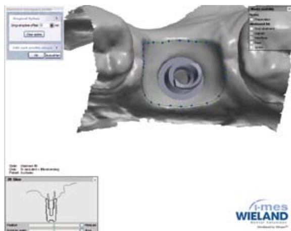
Fig. 11: Defining the transition between the build-up and the crown.
