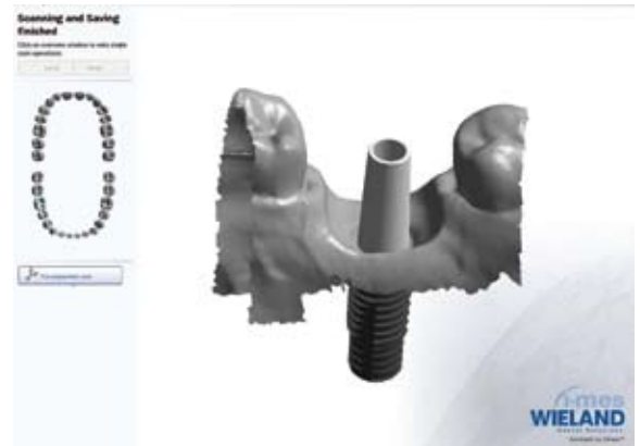
Fig. 10: Transfer of model situation using a scan build-up.
